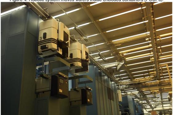
Figure 4. Robotic system moves wafers inside enclosed containers (FOUPs).
